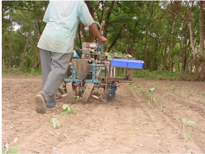
Fig. 16 Transplanting of brinjal by PTOVT using inclined press wheel
