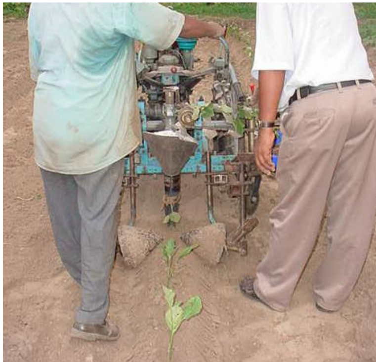
Fig. 17 Transplanting of brinjal by the machine using mould board and TCRS. (Transplanting and simultaneous ridging: Close-up view)
